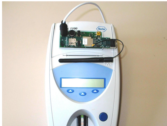
Figure 7.2: Urine Analyzer from Roche ® Diagnostics with Gumstix
